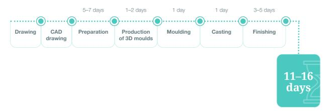
The centre's 3D printers will manufacture moulds for casting parts using material jetting technology by applying powder and gluing it with a binder.
